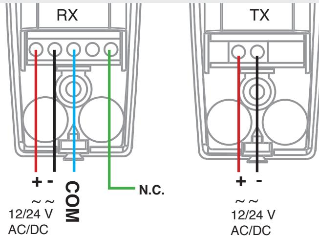
CABLAGGIO ALLA CENTRALE / WIRING ON CONTROL BOARD / CABLAGE SU LE CARTE
